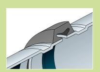
C-shape rubber gasket naturally seals on pipe ends.
