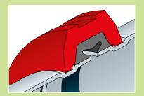
The housings compress the gasket to increase the sealing capacity.
